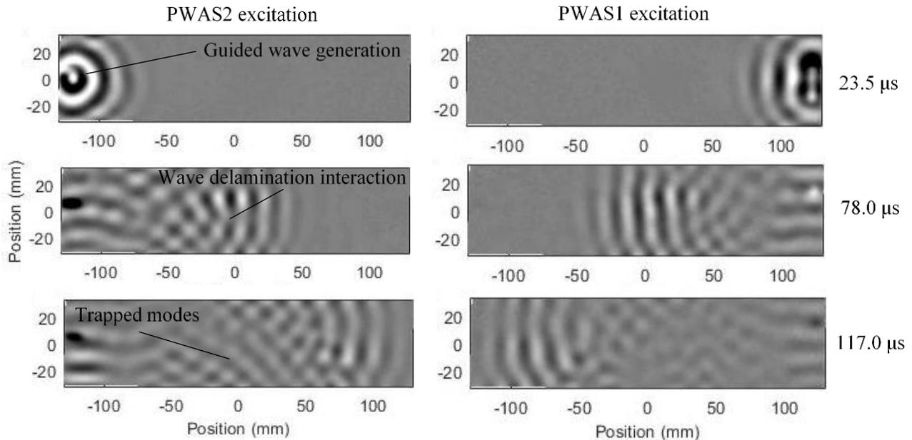
**FIGURE 7:** WAVE PROPAGATION IMAGE SNAP SHOTS FROM SLDV MEASUREMENTS
