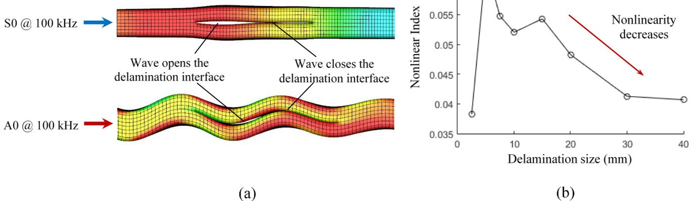
**FIGURE 5: DELAMINATION INTERFACE BEING OPENED AND CLOSED UNDER CYCLIC WAVE INTERACTION**
