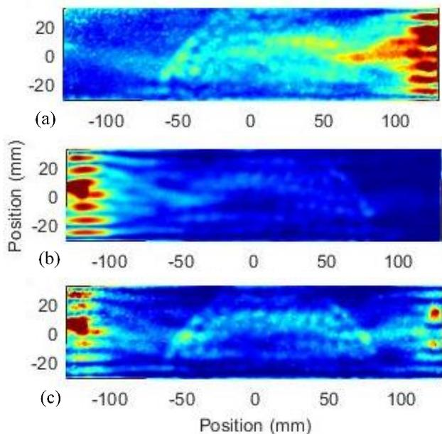
**FIGURE 8:** POST-PROCESSING IMAGING RESULTS FOR DELAMINATION QUANTIFICATION: (a) PWAS1 EXCITATION CASE IMAGE; (b) PWAS2 EXCITATION CASE IMAGE; (c) FUSED IMAGED FROM BOTH CASES
