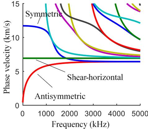
**FIGURE 3:** PHASE VELOCITY DISPERSION CURVE OF THE 4-MM THICK CARBON FIBER COMPOSITE PLATE
