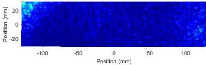
**FIGURE 10:** POST-PROCESSING RESULT FOR NONLINEAR WAVE FIELD DELAMINATION IMAGE
