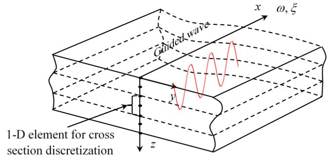
**FIGURE 1: SAFE MODEL OF WAVE PROPAGATION IN PLATE STRUCTURES**
