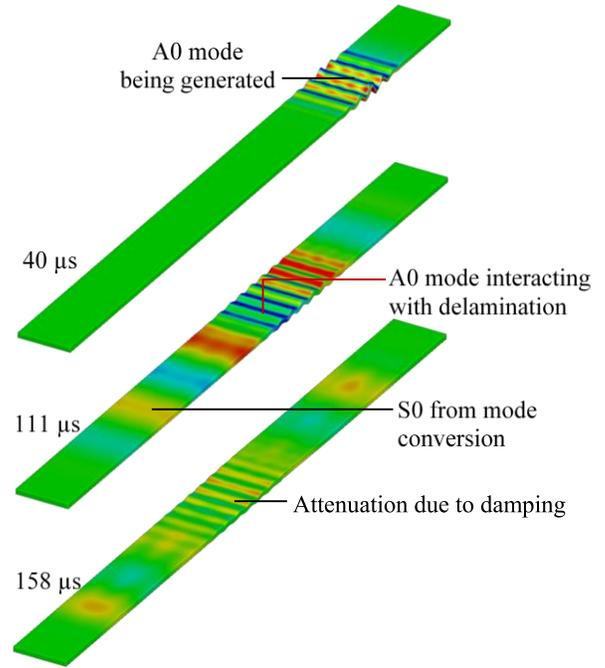
**FIGURE 4:** LISA SIMULATION OF WAVE PROPAGATION AND INTERACTION WITH DELAMINATION IN THE COMPOSITE PLATE
