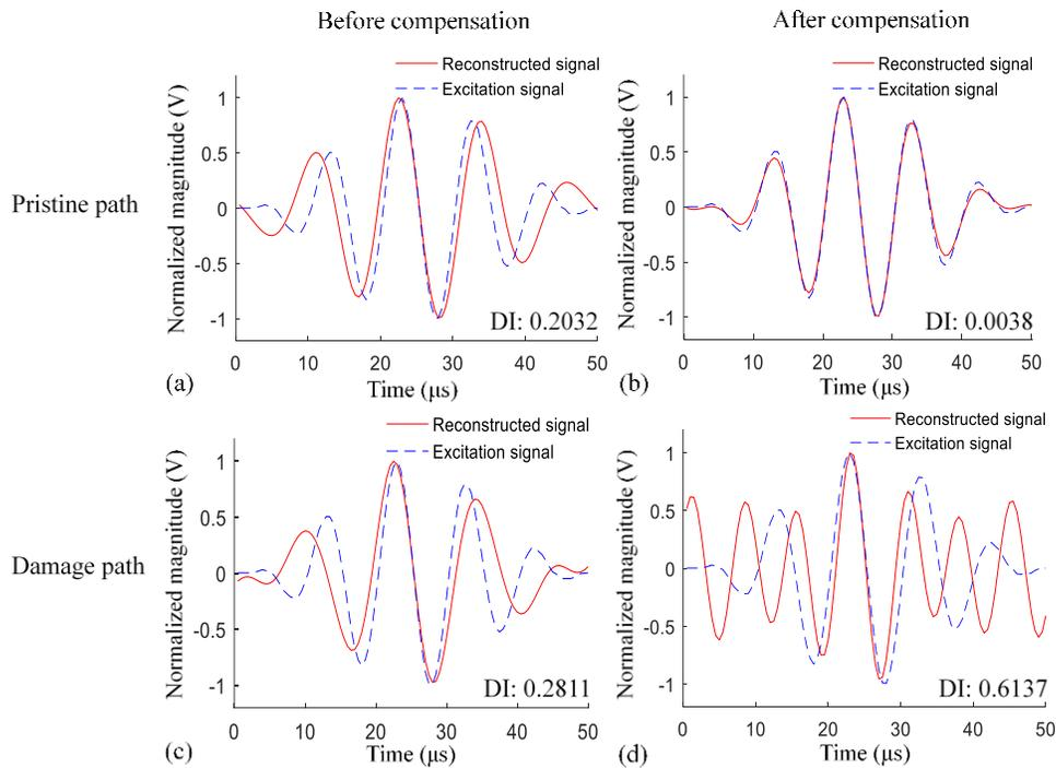
Figure 9. Reconstructed A0 signals: (a) pristine path before compensation (#16-#7); (b) pristine path after compensation (#16-#7); (c) damage path before compensation (#16-#6); (d) damage path after compensation (#16-#6).
