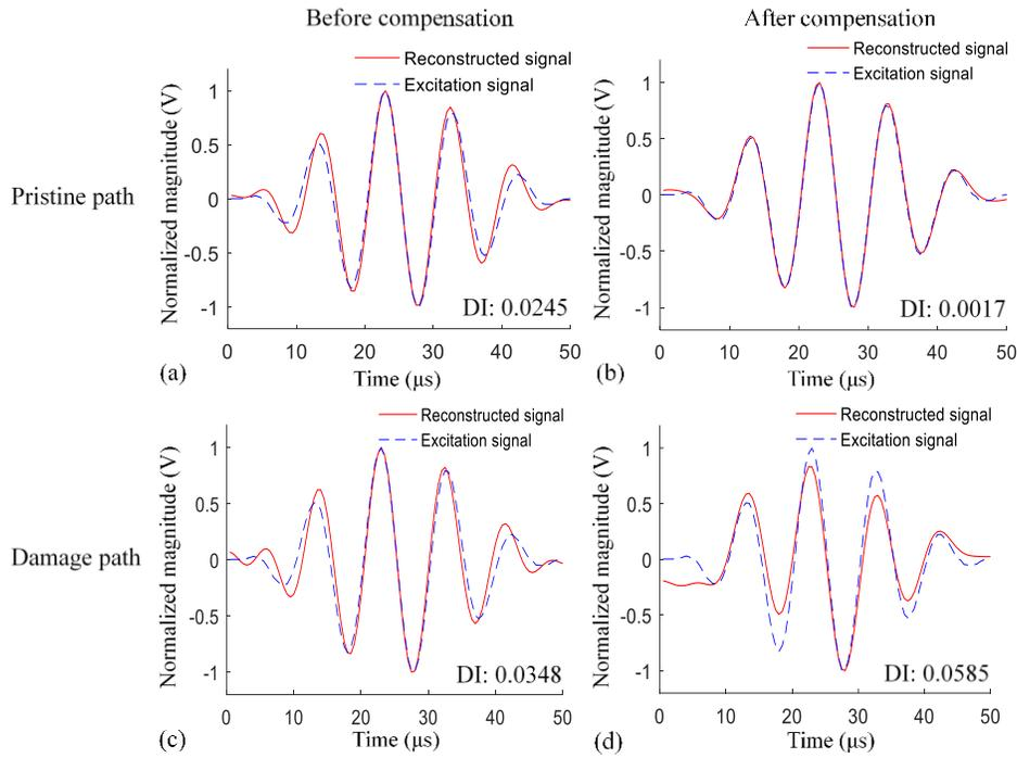
Figure 8. Reconstructed S0 signals: (a) pristine path before compensation (#6-#15); (b) pristine path after compensation (#6-#15); (c) damage path before compensation (#2-#10); (d) damage path after compensation (#2-#10).
