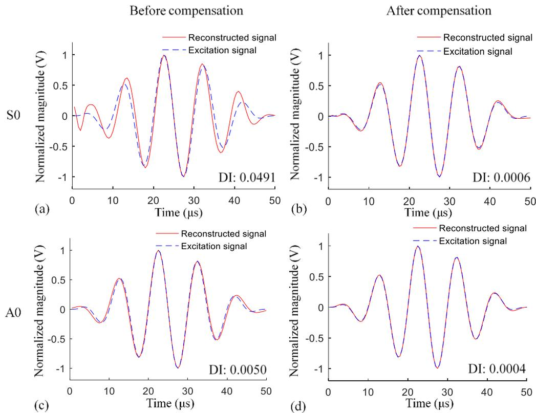
Figure 4. Virtual time reversal FE simulation results: (a) S0 mode before compensation; (b) S0 mode after compensation; (c) A0 mode before compensation; (d) A0 mode after compensation.
