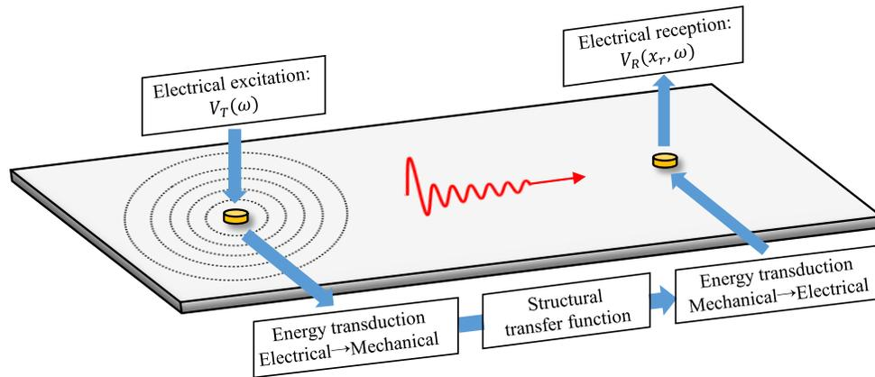
Figure 1. A typical pitch-catch active sensing procedure.
