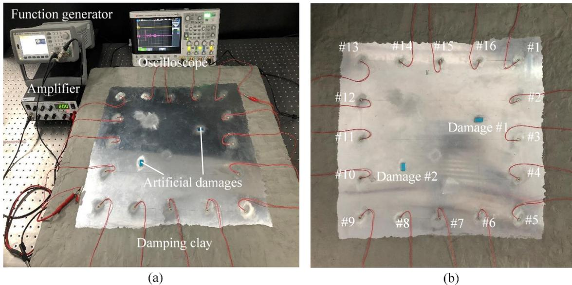
Figure 7. VTR damage imaging tests: (a) experimental setup; (b) specimen with a square active sensing PWAS array.
