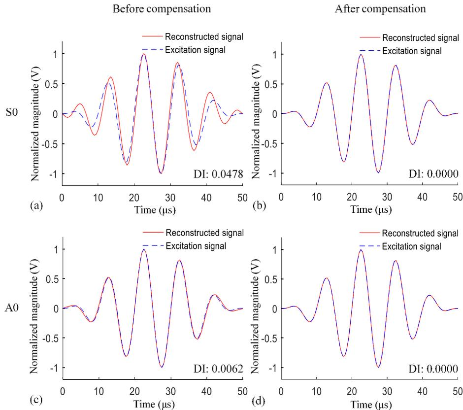
Figure 2. Virtual time reversal analytical results: (a) S0 mode before compensation; (b) S0 mode after compensation; (c) A0 mode before compensation; (d) A0 mode after compensation.
