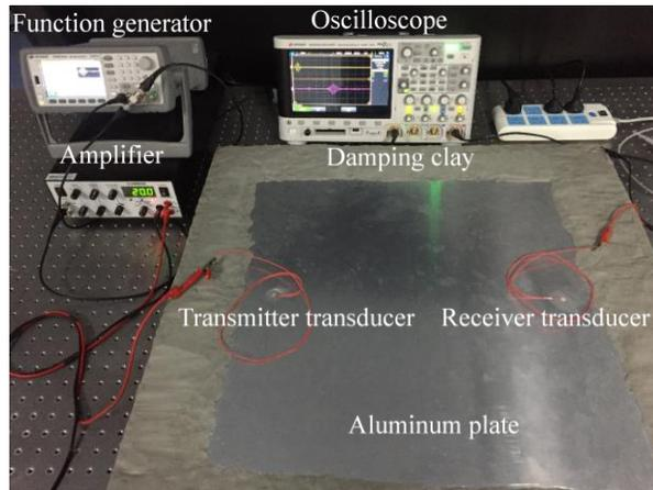
Figure 5. Experimental setup for pitch-catch active sensing.
