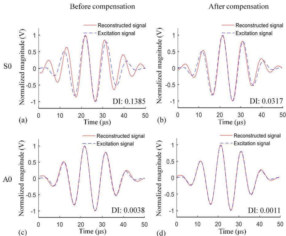
Figure 6. Virtual time reversal experimental results: (a) S0 mode before compensation; (b) S0 mode after compensation; (c) A0 mode before compensation; (d) A0 mode after compensation.
