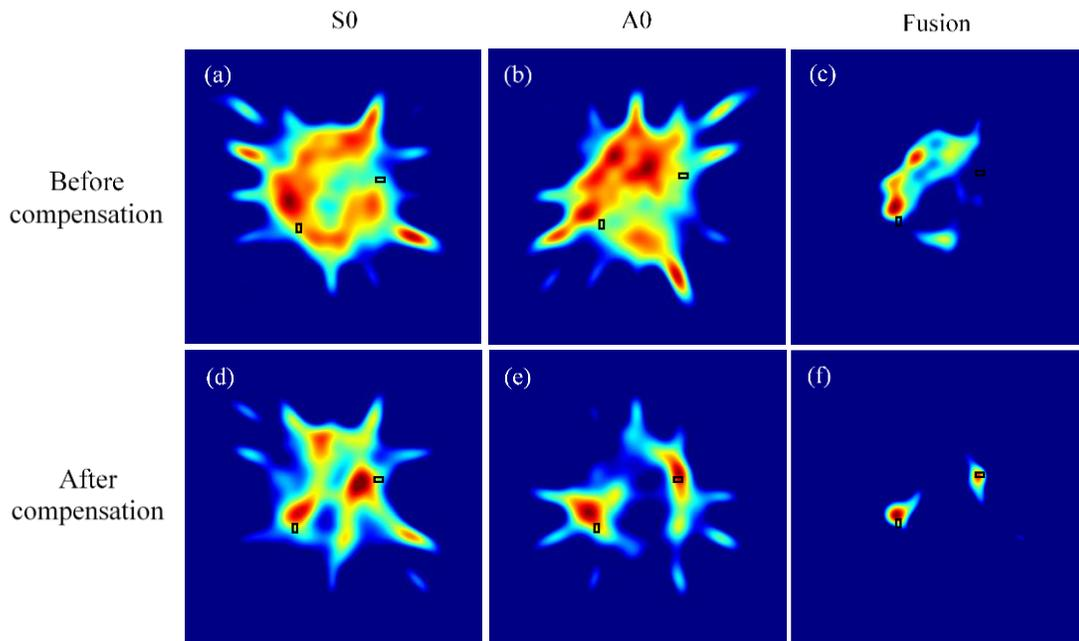
Figure 10. Damage imaging before and after compensation: (a) S0 summation tomography before compensation; (b) A0 summation tomography before compensation; (c) fusion tomography before compensation; (d) S0 summation tomography after compensation; (e) A0 summation tomography after compensation; (f) fusion tomography after compensation.
