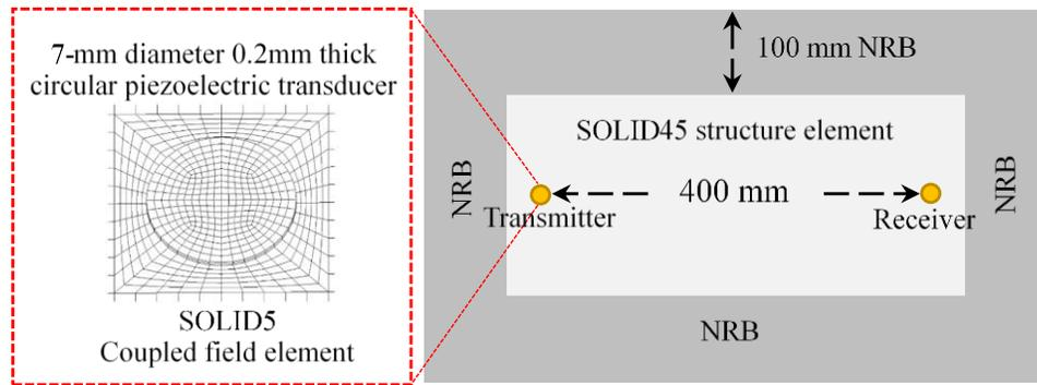
Figure 3. Finite element model for the pitch-catch procedure.
