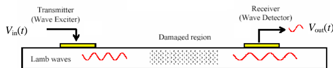
Figure 4 PWAS embedded NDE in pitch-catch mode as actuator and sensor
