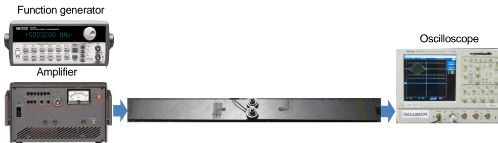
Figure 2: Experiment setup 1: pitch-catch active sensing using PWAS
