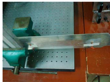
FIGURE 6. The aluminum plate clamped by a bench vice
